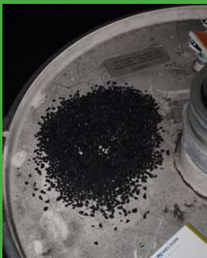
A sample of activated carbon on top of a MB recapture drum at Port Nelson
