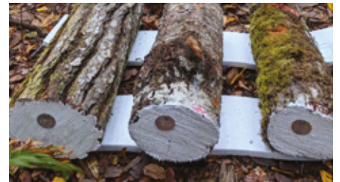
Three bolts each of Pseudotsuga menziesii , Pinus radiata , and Notholithocarpus densiflorus were placed at each field site. Bolts were elevated off the ground with styrofoam panels to avoid soil contact.
